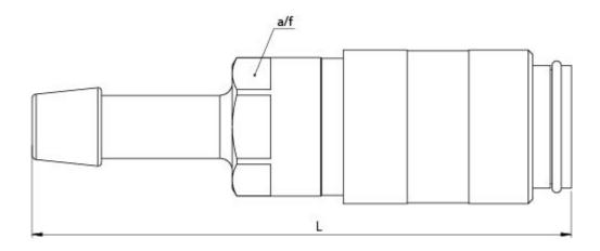
A/F = 19 Lenght = 160 Thread = M12x1 Tube diameter =  $\emptyset$ 8
